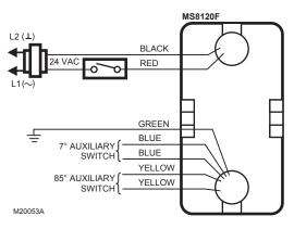
Fig. 6. Typical 24 Vac wiring (MS Series).
