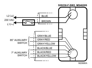
Fig. 10. Typical 230 Vac wiring (S20 Series).
