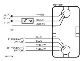
Fig. 7. Typical 120 Vac wiring (MS Series).
