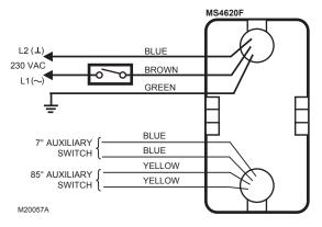
Fig. 8. Typical 230 Vac wiring (MS Series).
