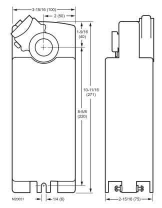
Fig. 1. Dimensional drawing of actuator in inches (mm).
