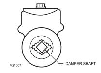
Fig. 3. Proper mounting to square damper shaft.
