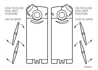
Fig. 2. Spring Return DCA mounting orientation.
